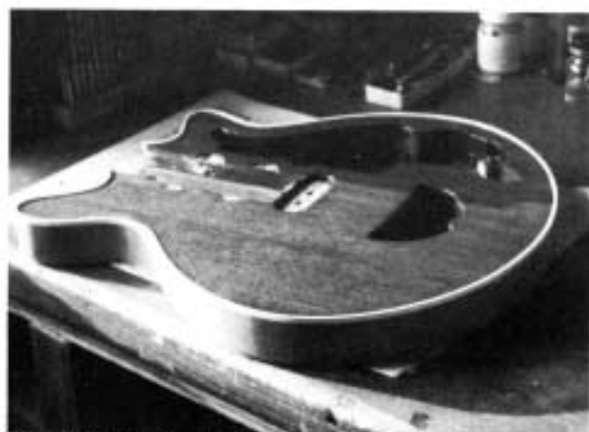
Body of Brian's guitar, showing acoustic pockets.
