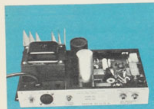
Solid-State component layout showing miniaturization and chassis compactness.
