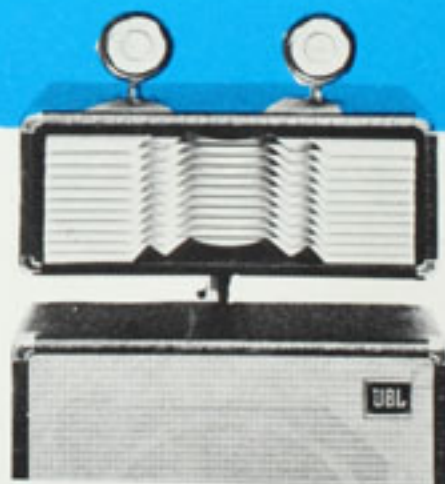
PAL 200 The most powerful mid-high frequency unit available. Includes two plug-in super tweeters response 800 - 20,000 Hz. High power crossover incorporated 180 watts R.M.S. 24 x 57 x 60 cm. 36 kg.
