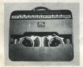
Output 60 watts. Two Special 12" Super Orbital speakers. Four inputs; two per channel. Channel One for solo, has Volume. 6-position Tone Selector, Treble, Vibrato Intensity and Vibrato speed controls. Channed Two has Volume and Treble controls. On/off switch and indicator lamp, Vibrato operated by heavy duty foot switch. Operation on 200/250v., a.c. 40/60 c.p.s. or 100/ 150v., a.c. 40/60 c.p.s. both with automatic adjustment. Size 21" high, 25" wide, 10" deep.
